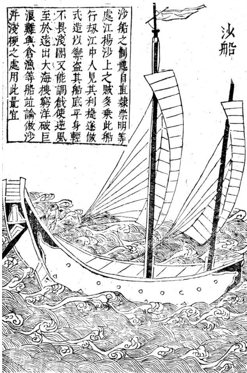
Figure 12. Picture of sandboat, 1646. This woodblock print depicts a sandboat, a sturdy vessel that Zhang Huangyan used when launching his assault of the “Roiling River Dragon” in 1659. The text on the left notes that “the bottom is flat, and the body is light, so that it fears no shallows. It can be employed to go upwind, for it defies the wind.” On these sandboats, Zhang Huangyan sailed swiftly up the Yangtze, well in advance of Koxinga’s main fleet. From Zheng Dayu, Jing guo xiong lue , “Wu bei kao,” juan 18, quote from folio 7v. Used by permission of Harvard Yenching Library.
